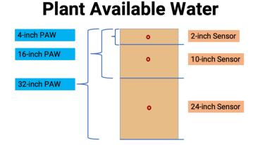
The diagram on the left shows the location of the 2-inch, 10-inch, and 24-inch soil moisture sensors. The 4-inch PAW uses data from the 2inch sensor. The 16-inch PAW uses data from both the 2-inch and 10-inch sensors. The 32inch PAW uses all three sensors with the deepest sensor at 24 inches.
