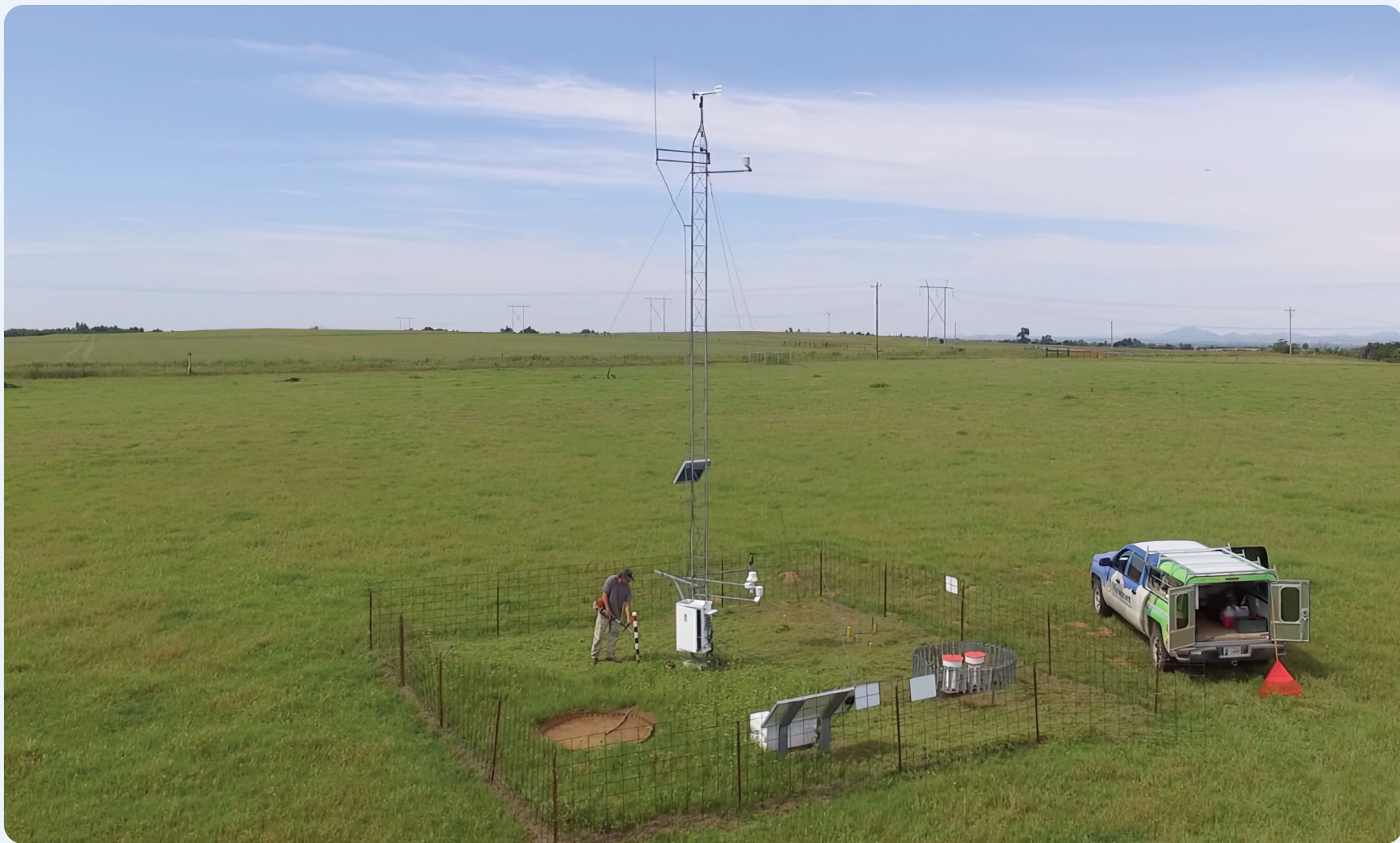
Oklahoma Mesonet sites are visited multiple times each year by highly trained technicians to maintain the highest possible data quality. In this aerial photo from June 2017 , a Mesonet technician performs routine summer vegetation maintenance at the Oklahoma Mesonet site in Apache, OK . (Photo by Chris Fiebrich)
